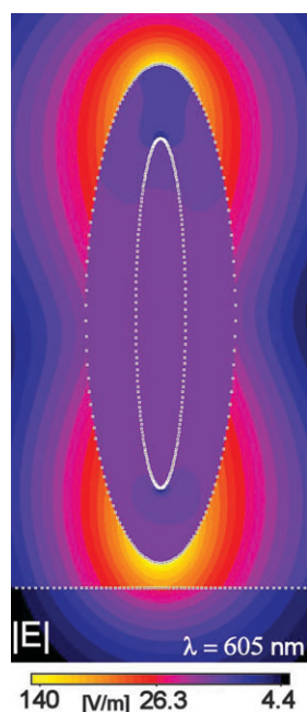
Fig. 2 MMP calculation of the field distribution of an evanescently excited ellipsoidal particle with a glass core.
